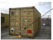
Container seals have to be fitted at the right container door - the inner locking bar /handle- only. Or as shown right
